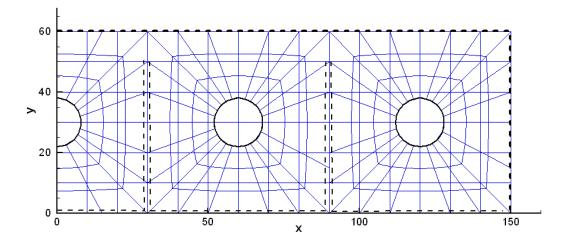
Figure 14.2: View from above the free surface showing one quadrant of the control surface described in Example 4. The rectangular outer boundary and partition boundaries are represented by the heavy dashed lines. Gaps between the partition boundaries are included for clarity, and are not present in the CSF file.
