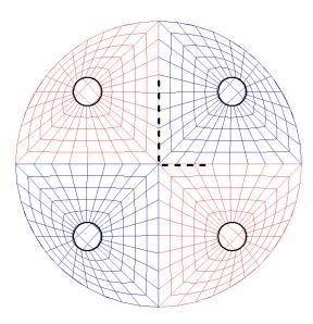
Figure 14.1: View from above the free surface showing four quadrants of the TLP control surface with a circular outer boundary. The partition boundary is represented by the heavy dashed line, as input in the CSF file shown above for Example 3, before it is extended by the program to intersect the outer boundary.
